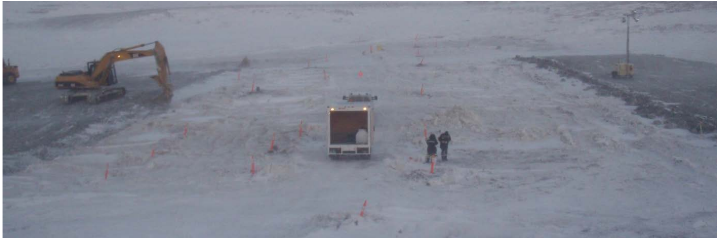
Approximate north-northeast view towards percolation testing. Note the heated cube truck in the center of the photo was used to hold testing equipment and maintain water temperatures around 10-20 °C, January 29, 2011
