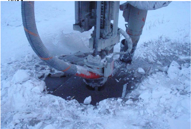
Drilling and collecting soil sampled from percolation hole P24, January 28, 2011
