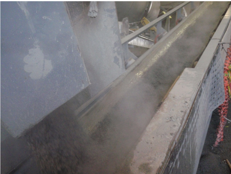
Moisture-conditioned core material exiting the chute, March 23, 2011
