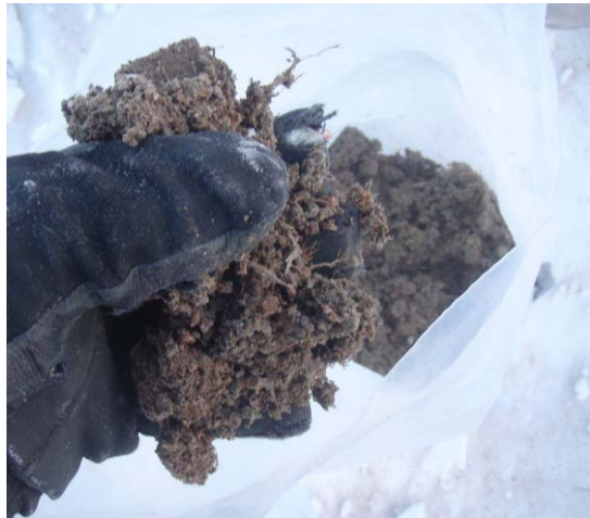
Example of organic rich soil (peat) encountered at ~1.5 m depth in percolation hole P04 January 24, 2011
