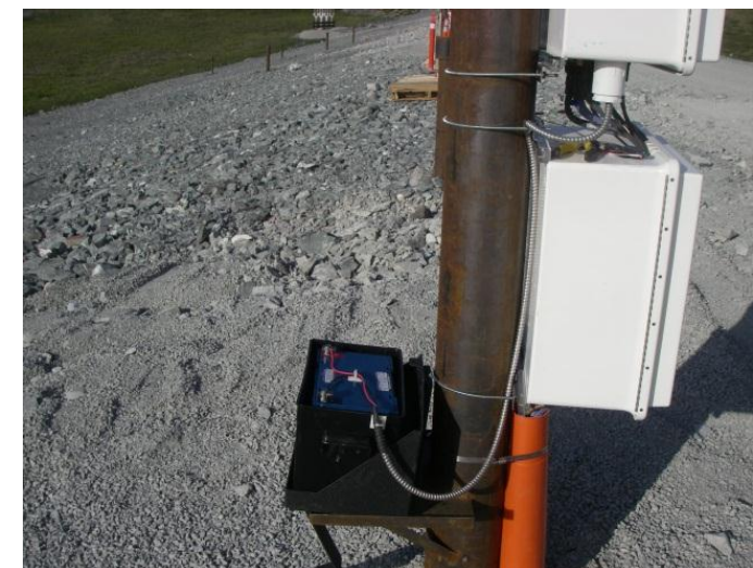
Typical instrument support post setup. The instrumentation housing on top, the cable management box underneath, and the battery on the back side.
