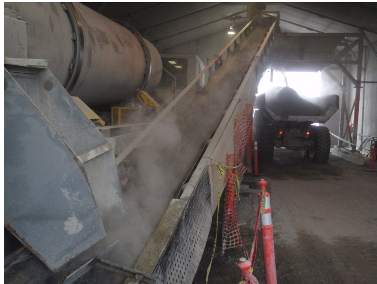
Frozen Core Plant chute and conveyor belt in foreground, surge bin and loaded truck in background, photo taken March 31, 2011
