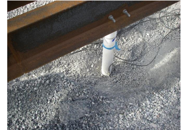
Thermosyphon status thermistors were attached to thermosyphon risers using epoxy resin and zip-ties.
