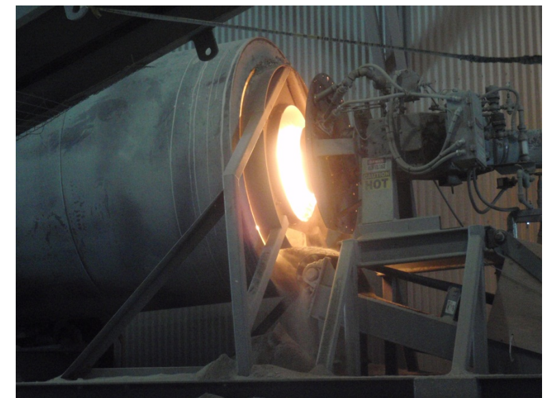
The flame at the top end of the drum heats the dry core material, May 2, 2011
