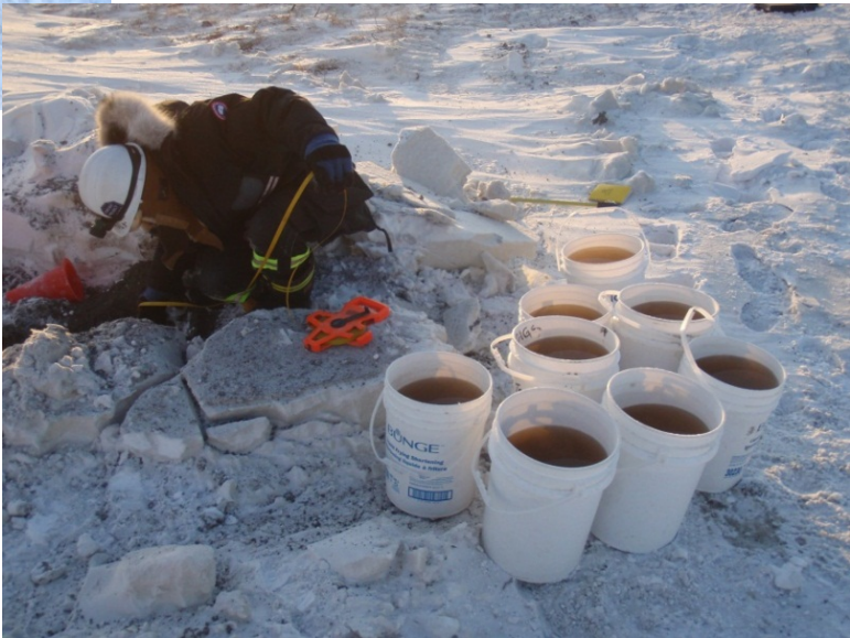
(Right) Rechecking drilled percolation hole depth before final stage of testing, February 1, 2011
