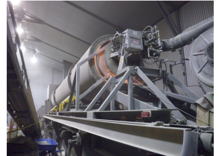
Drum in which the dry core material is heated and mixed with water to form the moisture-conditioned core material, March 9, 2011
