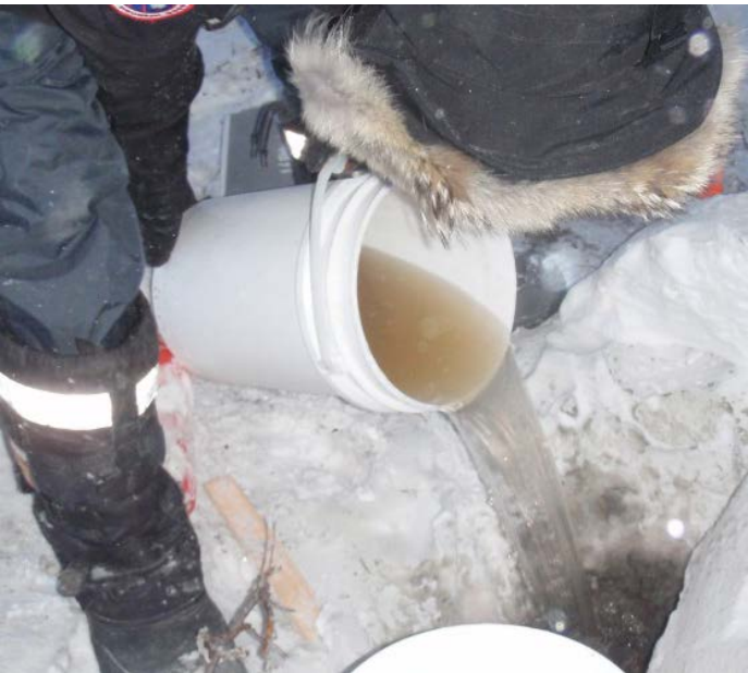
Pouring warmed water from Doris Lake into percolation hole, January 30, 2011
