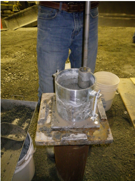
Standard Proctor testing, March 5, 2011
