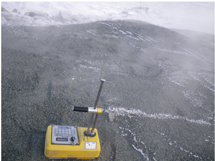
In-situ density testing of freshly placed core material with Troxler Gauge, February 27, 2011
