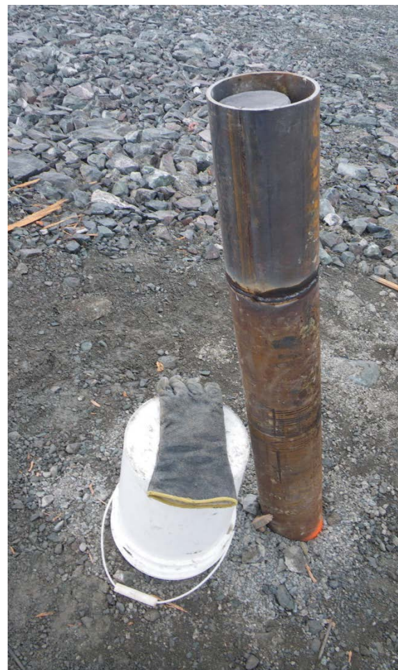
Completed deep settlement point installation, May 6, 2012
