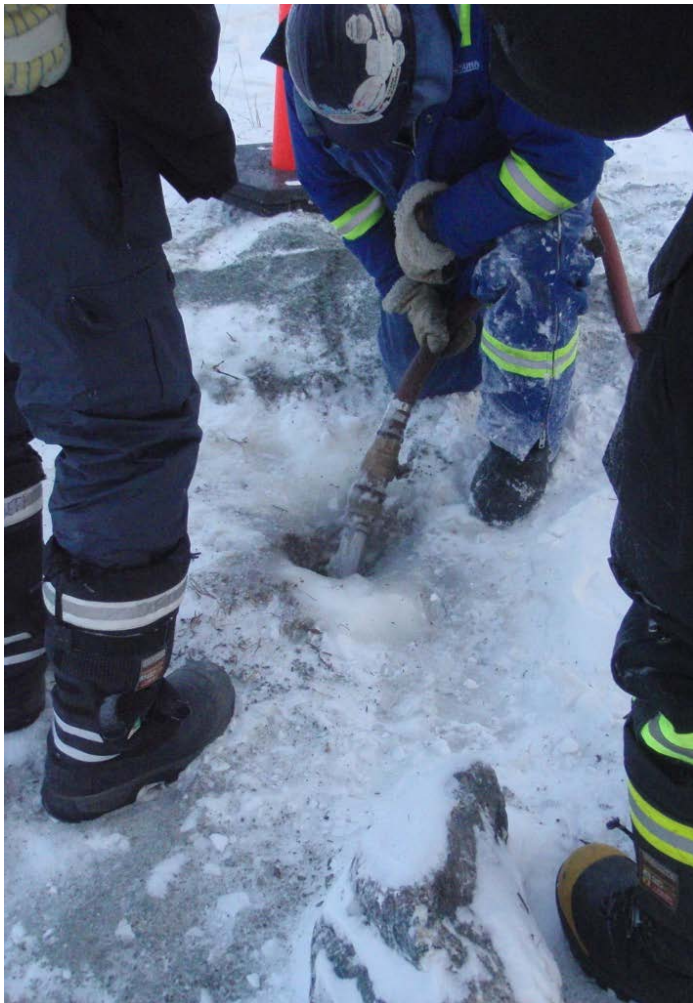
Initial attempt at completing percolation testing with hose from water truck, January 28, 2011
